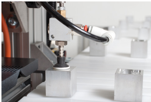
Multi-position loader that permits a continuous production cycle.
